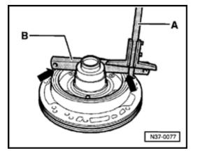
Place straightedge "B" onto stator support (-arrow-) and measure with depth gauge "A" to gasket of pump flange.
