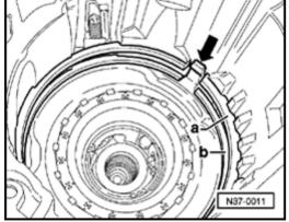
Preload free wheel rollers with 3267 assembly ring and install free wheel.
