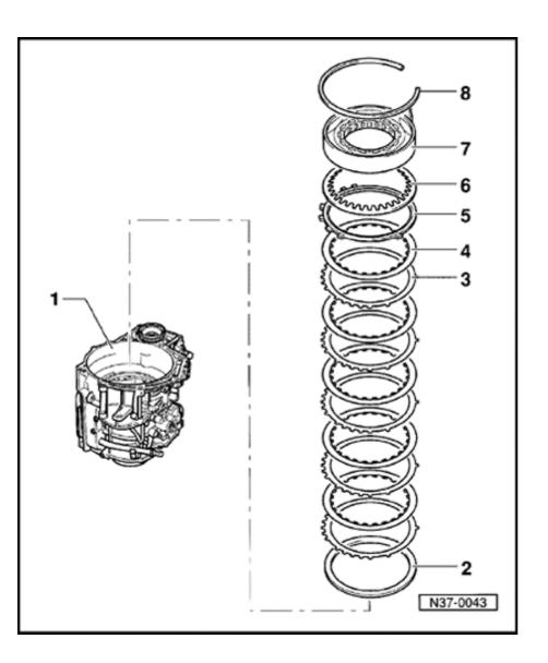
Reverse gear brake -B1-, adjusting
