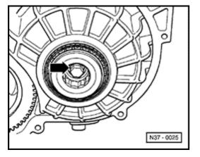
Insert screwdriver through hole of large drive shaft and large sun gear to loosen and tighten bolt for small drive shaft.
