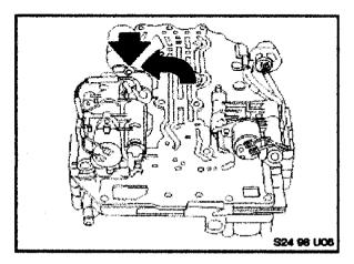
Put a dot of green paint on the transmission control unit plug after it has been checked and/or corrected.
