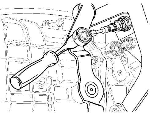
12. Release the support bracket sleeves (press tabs in the direction indicated by the arrow) and carefully pull them out of the bracket.
