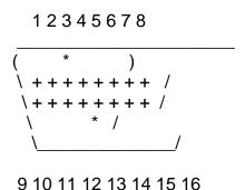
Using the jumper wire connect the - ground to the ENGINE CONTROL or jumper the OBD-II connector
